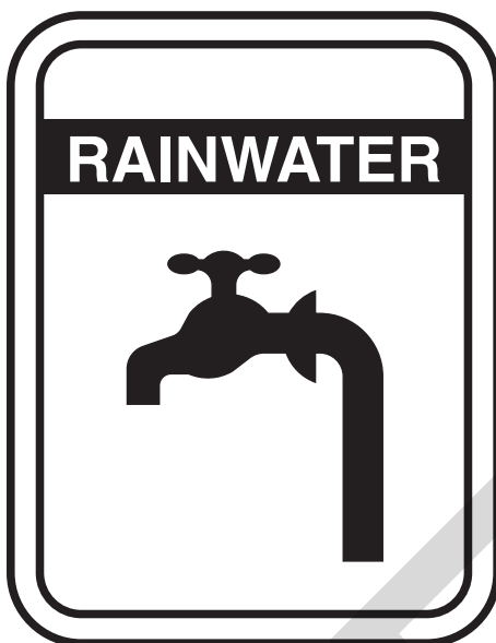
FIGURE 16.3.2.2 TYPICAL SIGN FOR RAINWATER OUTLETS
